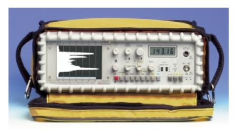
1/3 of the band in use to approx. zero). In the Monitor mode, the instrument demodulates the analog TV signal, which enables a terrestrial or satellite television channel to be identified and its reception observed. The signal level in monitor mode is represented by an analog bar at the top of the image. The bar length varies in proportion to the power received. In addition it enables the line synchronism pulse to be observe on the top center of the screen.
